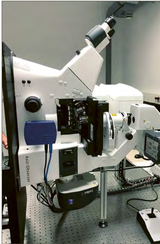
Figure 2: Our vertically-oriented confocal microscope for the long-term high-resolution imaging of plant-microbe interactions
