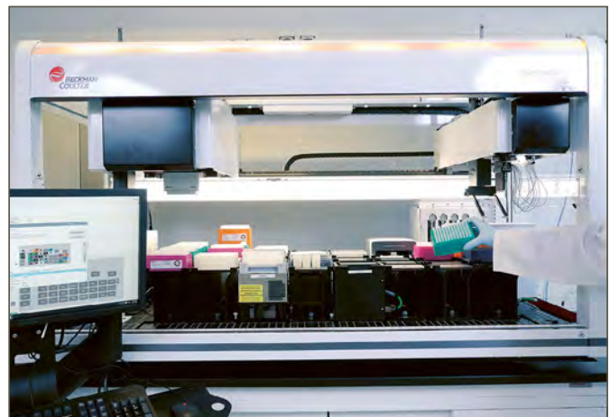
Figure 1: NGS library preparation by robotics. High-throughput library preparation for NGS at MP-GC is routinely performed by robotic systems such as the Biomek i7 in a 96-well scale to minimise hands-on time and reduce the variation associated with liquid handling. The MP-GC tailors existing protocols and designs new ones if required.
